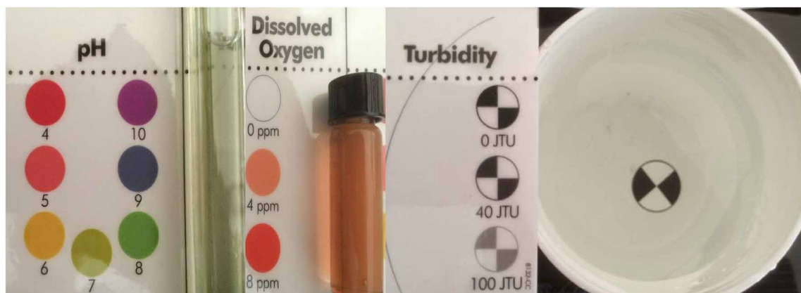
Figure 4. World water monitoring challenge kit (EarthEco International, 2015)
