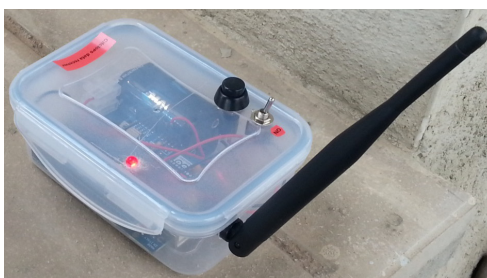
Figure 4: Receiver based on an Arduino platform
