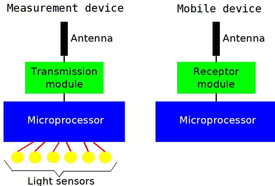
Figure 2: Basic modules of the low cost system
