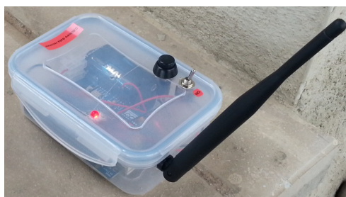
Figure 4: Receiver based on an Arduino platform
