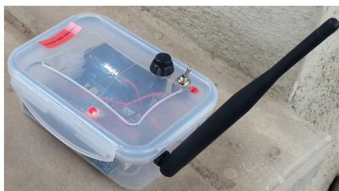
Figure 4: Receiver based on an Arduino platform
