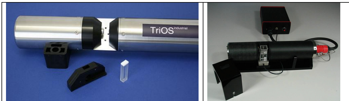
Figure: Cuvette holder for portable absorption device (ProPS, TriOS) 1 and workstation for bbe's FluoroProbe 2 . The FluoroProbe without workstation is in the highest price range of > 10,000 EUR.
